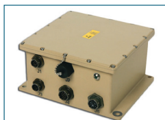
Figure 1 | The upgraded OBC embedded computer needed to fit within an existing sealed enclosure
