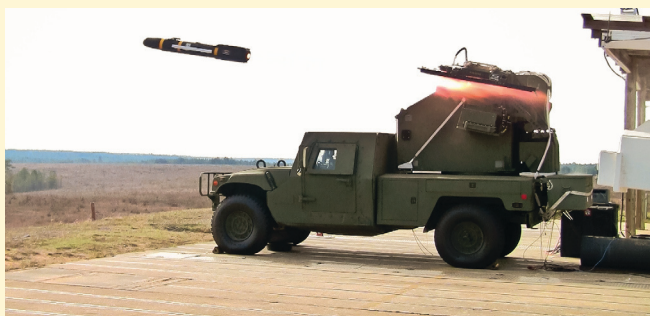
Figure 3 | Boeing recently supported the U.S. Army's initial test launch of a modified Avenger turret-fired AGM-114 Hellfire missile at Eglin AFB. Photo courtesy of U.S. Army
